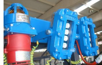
All circuits and components are located in a flameproof enclosure.
