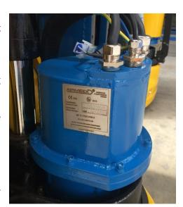
All circuits and components are located in a flameproof enclosure.
