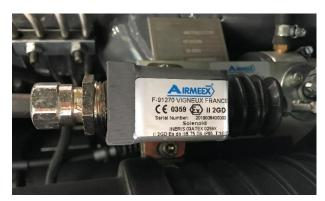
All circuits and components are located in a flameproof enclosure.
