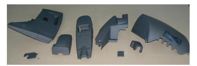
Plastic parts on which the operator is frequently or constantly in contact with the vehicle have been made antistatic due to the risk of electrostatic and are protected with special paints.
