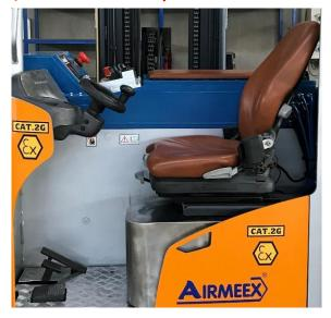
As part of a daily work, the condition of the above-mentioned parts should be checked visually. In the event of any wear or antistatic condition on the parts, the vehicle should not be used and Airmeex authorized personnel should be contacted immediately.
