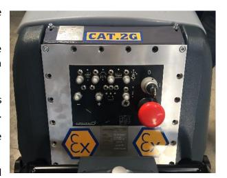
The functional buttons and buttons on the vehicle are replaced with Ex equipment suitable for use in a hazardous area. It allows the operator to manage the vehicle by using 'd' type on a flameproof enclosure. It differs visually from the buttons and buttons used by the original equipment manufacturer. The definitions on the vehicle regarding the duties of the buttons and switches should be taken into consideration.
