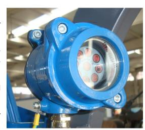
All circuits and components are located in a flameproof enclosure.
